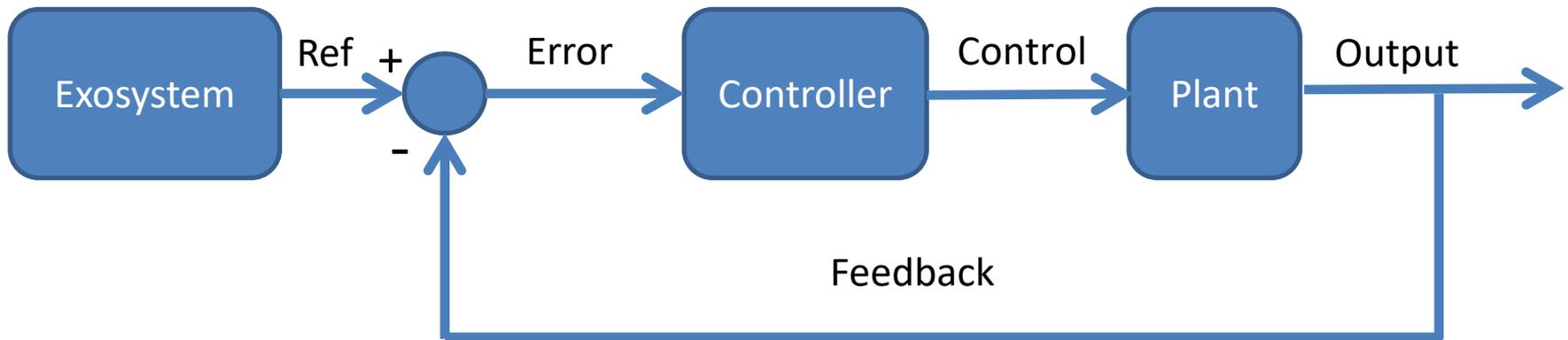
Total system = (Exosystem, Controller, Plant) =  $\mathbf{S} = (X, \alpha)$
