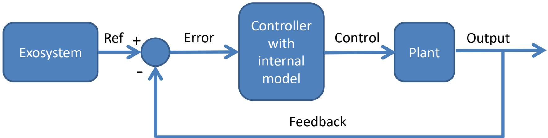
Total system = (Exosystem, Controller, Plant) =  $\mathbf{S} = (X, \alpha)$
