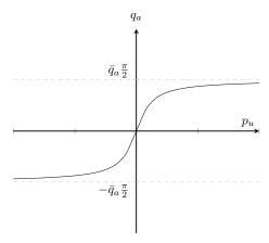
Fig. 2: The acrobot constraint  $q_a = \bar{q}_a \arctan(Ip_u)$ .
