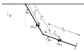
Fig. 4: The distributed mass acrobot model, represented by two weighted rods differing in both length and mass.
