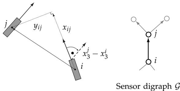
Fig. 2. Illustration of the relative kinematic variables sensed by unicycle  $i$  if there is an edge from node  $i$  to node  $j$  in the sensor digraph.
