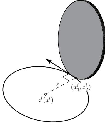
Fig. 3. The centre of rotation  $c^i(x^i)$  of unicycle  $i$  if  $|x_5^i| > 0$  and  $x_4^i = x_5^i/r$ .
