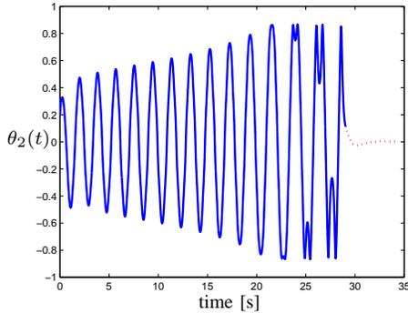
Fig. 7. Angle  $\theta_2(t)$  for the pendubot example.
