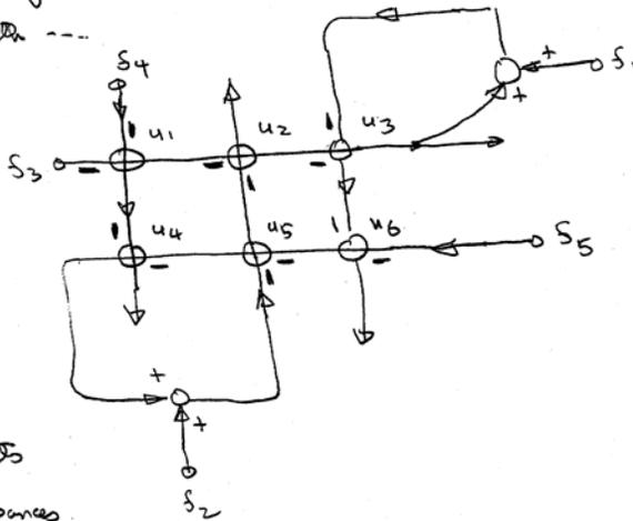
Want to control queue lengths of travel in NS & EW direction. In this figure there are 6 inputs 12 outputs & 5 disturbances
