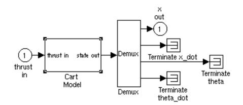
where "thrust in" is the input u of the nonlinear differential equation, and "state out" is the solution of the nonlinear state equation. This block corresponds to the nonlinear state equation and is a subsystem of the simulink model. It can be built in the form described by the following figure:
