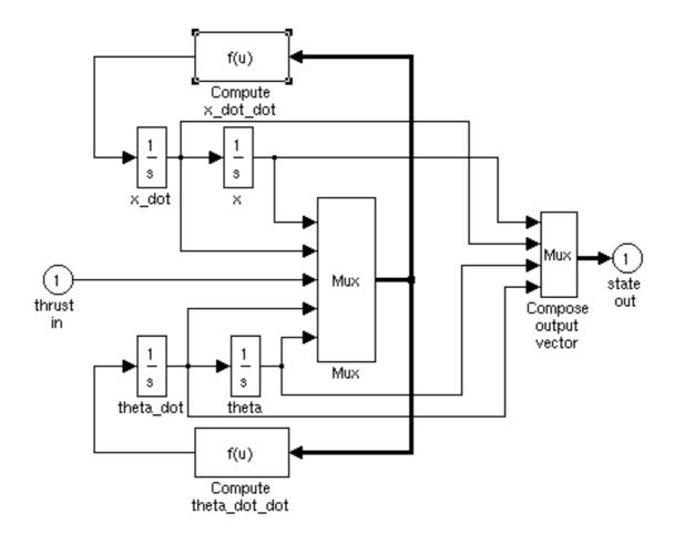
For blocks from the User Defined Function Library are used to specify the nonlinear functions in the system (denoted f(u) in the figure). Since the nonlinear functions are complicated, use of the For blocks is strongly recommended. Based on these suggestions, set up the complete simulink model corresponding to the inverted pendulum on a cart system. Save your complete model in simulink as, say, invertpen.mdl. Write down the 2 nonlinear functions and the complete f(x, u)in the space below:
