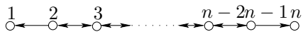
Fig. 6. The sensor digraph for a group of wheeled vehicles with two edge leaders.
